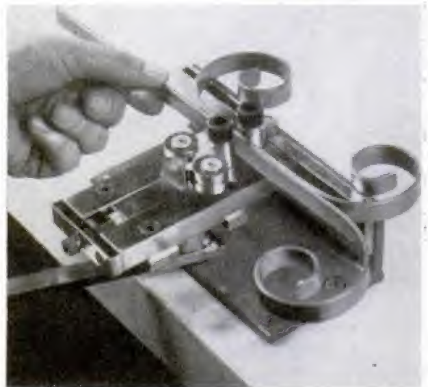
RIVETER-FORMER squeeze-sets rivets against anvils held by Allen-head screws when lever is pulled hard
